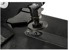
Position strut, spikes up, on spring pegs
