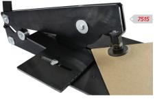
Place backing board in PG-28. Adjust back gauge to give suitable position for pressure pad
